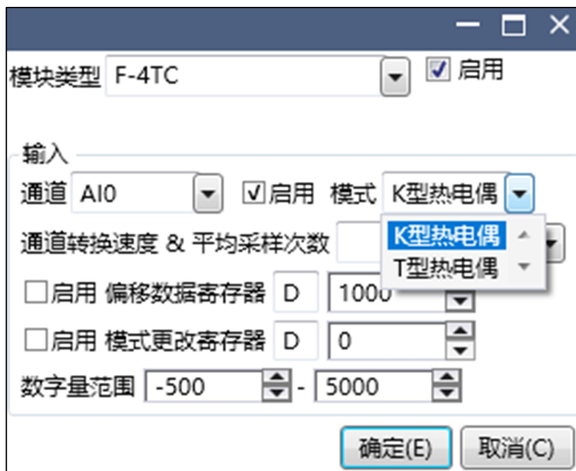
Figure 2.10: Expansion Plugin F-4TC Configuration Parameters
