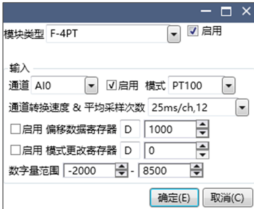
Figure 2.11: Extension Plugin F-4PT Configuration Parameters
