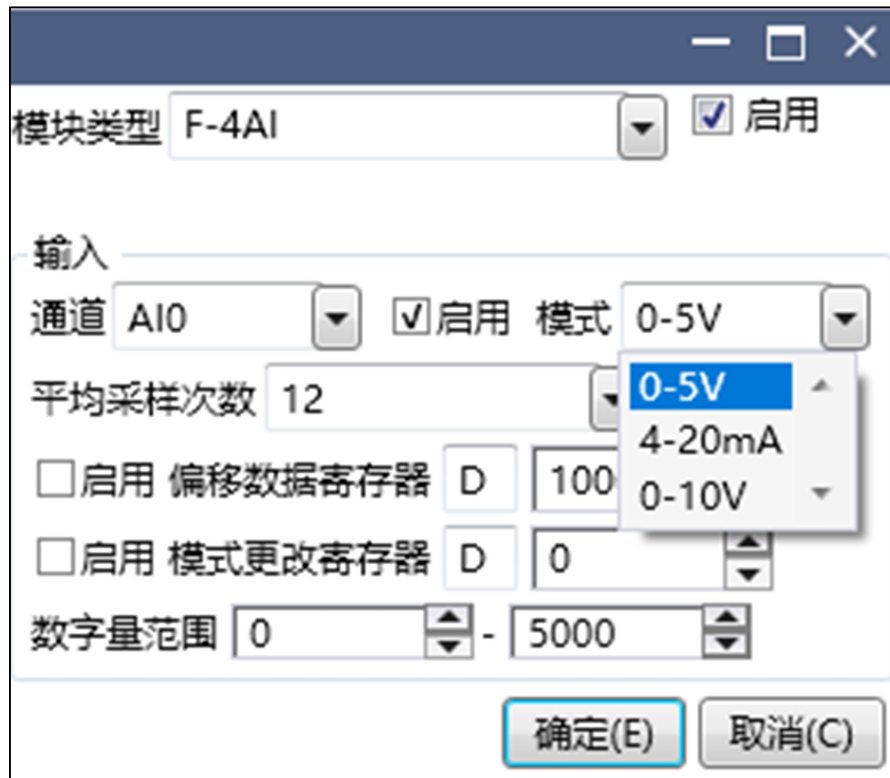
Figure 2.8: Extension plug-in F-4AI configuration parameters
